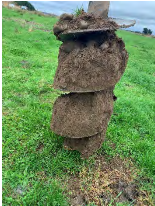
Left image: Site ORSL_2 at 0.5 m depth shows similar soil throughout suggesting it has not been disturbed previously.
