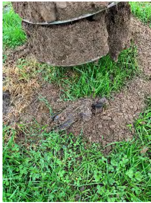
Left image: Site ORSL_2 at 0.5 m depth shows similar soil throughout suggesting it has not been disturbed previously.
