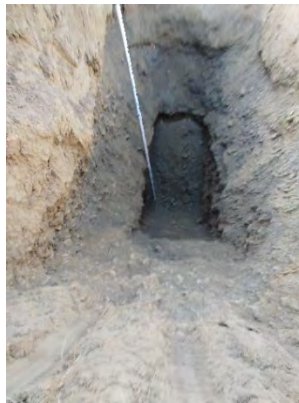
Left image: Site ORSL_2 at 3.5 m depth. No rubbish is seen in the drill flights and the soil is similar throughout suggesting it has not been disturbed.
