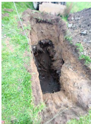
Left image: Site TP235 showing a sudden change in soil colour indicating there may have been disturbance at some point in time.
