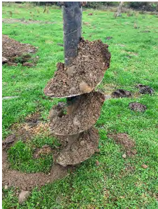
Left image: Site ORSL_2 at 3.5 m depth. No rubbish is seen in the drill flights and the soil is similar throughout suggesting it has not been disturbed.
