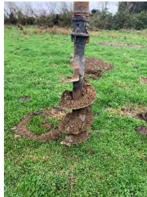
Left image: Site ORSL_2 at 0.5 m depth shows similar soil throughout suggesting it has not been disturbed previously.
